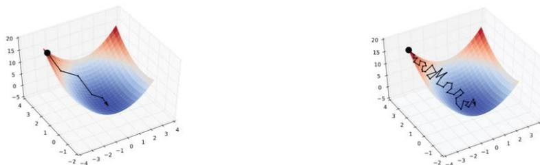
Figure 4: Visualizing the convergence pattern of BGD (left) and SGD (right) to a single minimum in dark blue<sup>[1]</sup>.
