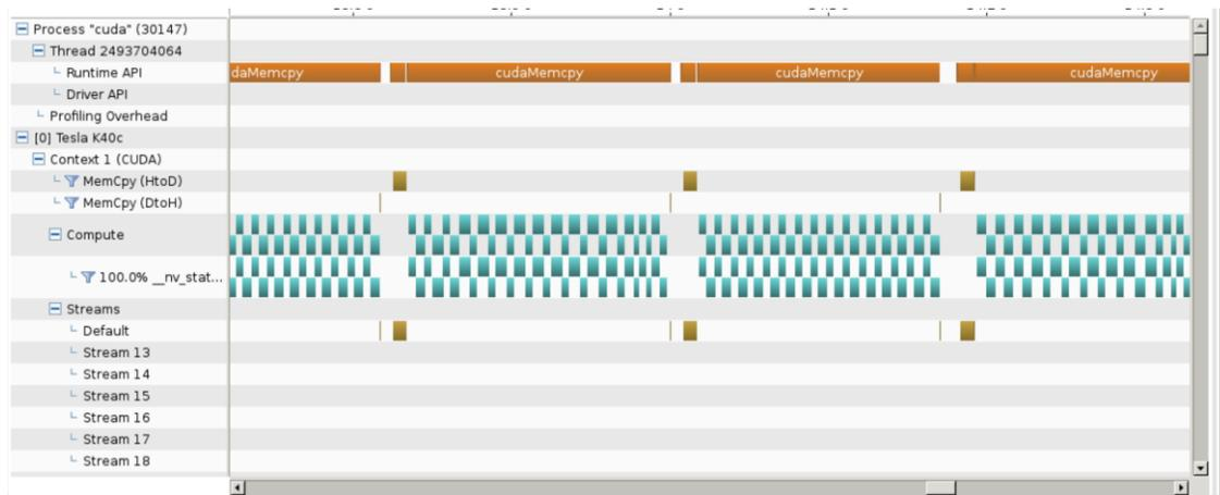
Figure 13: Timeline output of NSight: 10ms memcpy, 3.5ms per kernel call
